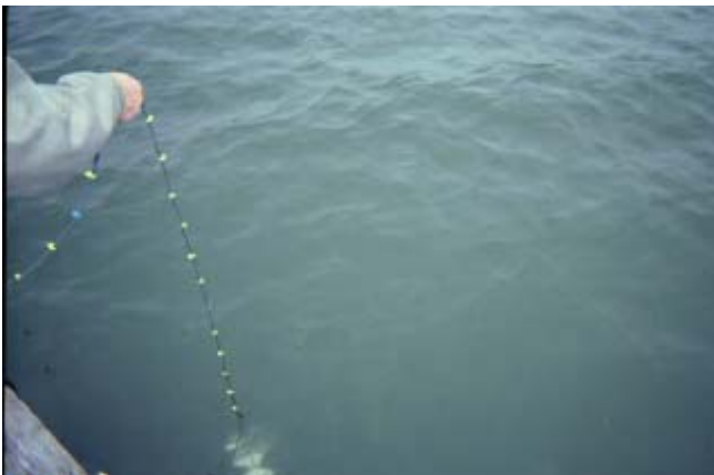
A volunteer monitor measures water clarity with secchi disc.
