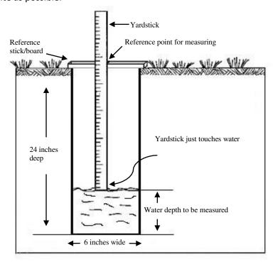
**Step 5:** Check the next day to make sure that the second filling has drained within 24-36 hours. An optimal infiltration rate is 1.2 inches per hour and minimum acceptable infiltration rate is .3 inches per hour – **if the hole has not drained within 36 hours a rain garden or permeable paver project is not possible.**
